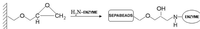
Fig. 1. Schematic illustration of the covalent method for the enzyme immobilization on Sepabeads EC-EP support
