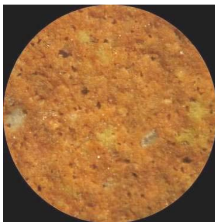
Slika 7. Snimak betona na bazi reciklirane šamotne opeke na optičkom mikroskopu Figure 7. Micrograph of concrete based on recycled shamote obtained using the optical microscope
