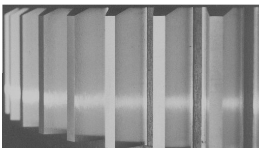
Figure 4. Hardfaced and finished gear geometry: circular pitch diameter \varnothing 258 mm, correction factor x_m = 0 , root diameter \varnothing 244.8 mm, working length of teeth 40 mm, pitch line 18.84 mm. Slika 4. Tvrdo navaren i poliran zupčanik sa geometrijom: prečnik podeonog kruga \varnothing 258 mm, korekcionni faktor x_m = 0 , prečnik korena zubaca \varnothing 244.8 mm, radna dužina zubaca 40 mm, hod spreznjanja 18,84 mm
