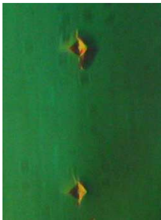
Fig.1. Uncoated substrate of silicon; Evidence of brittle response during indentation on Si(100) at 0.392 N load. The diagonals were parallel with \langle 110 \rangle orientations.
