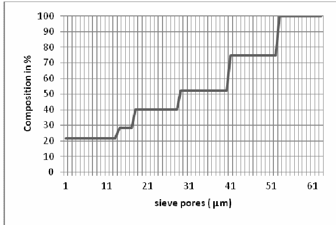
Fig. 4. Granulometric composition of the slag sample
