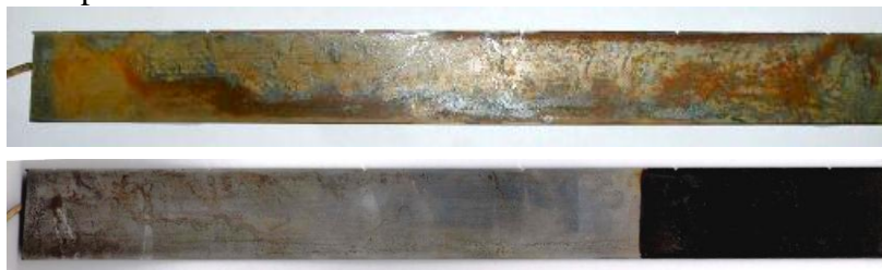
Figure 9. Comparison of the images of bare mild steel and mild steel with partial PANI-benzoate coatings after a ten-hour exposure to 3% NaCl at the corrosion potential.
