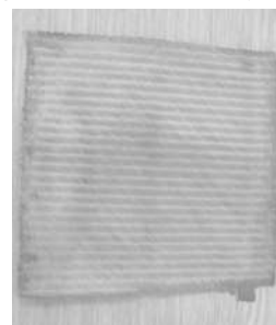
Figure 4- Colon fabric impregnated with 1.0 wt.% MWCNT/PVB/ethanol solution
