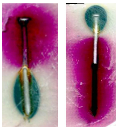
Fig. 16. Ferroxy indicator test of an unprotected (left) and a PANI-protected nail (right) after 10 h.
