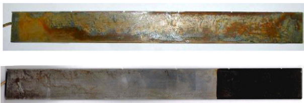
Fig. 11. Comparison of the images of bare mild steel and mild steel with partial PANI-benzoate coatings after a 10-hour exposure to 3% NaCl at the corrosion potential.
