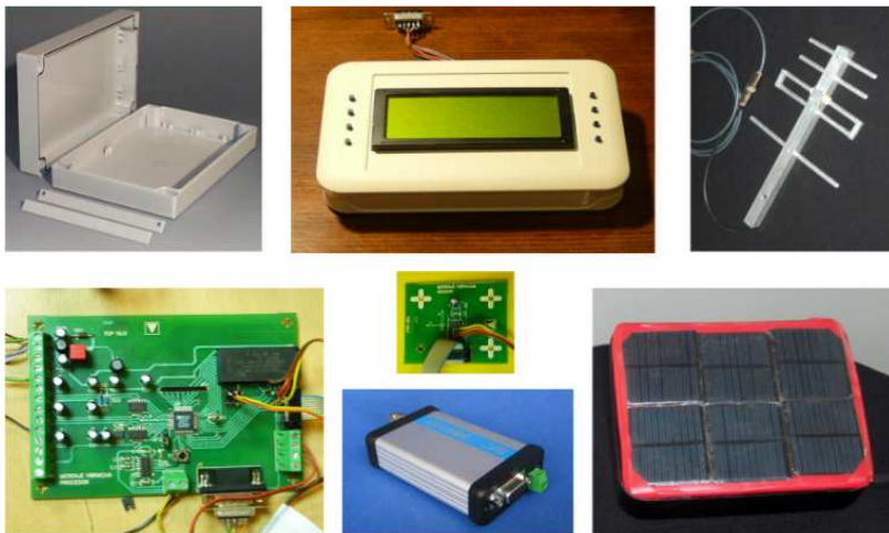
Fig. 1. Parts of the sensor device: the housing, LCD, the Yagi antenna, the boards, the radio modem, and the solar panel.
