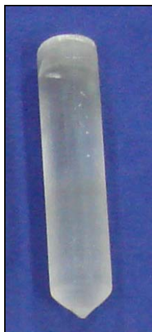
Fig. 2. Photographs of Bridgman-grown \text{CaF}_2 single crystal.
