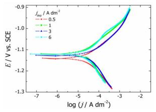
Figure 3. Polarization curves in 3% NaCl for Zn-Ni-Co alloy coatings deposited at different current densities from sulfate bath, [Co<sup>2+</sup>]/[Ni<sup>2+</sup>] = 0.1
