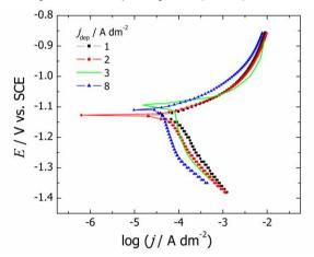
Figure 1. Polarization curves in 3% NaCl for Zn-Ni-Co alloy coatings deposited at different current densities from chloride bath,  $[Co^{2+}]/[Nf^{2+}] = 0.1$ .
