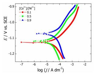
Figure 4. Polarization curves in 3% NaCl for Zn-Ni-Co alloy coatings deposited at 3 A  $dm^{-2}$  from sulfate bath at different [Co<sup>2+</sup>]/[Nl<sup>2+</sup>] ratios
