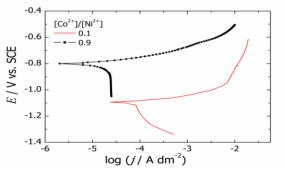
Figure 2. Polarization curves in 3% NaCl for Zn-Ni-Co alloy coatings deposited at 3 A dm<sup>-2</sup> from different [Co<sup>2+</sup>]/[Ni<sup>2+</sup>] ratios
