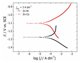
Figure 5. Polarization curves in 3% NaCl for Zn-Ni and Zn-Co alloy coatings deposited at 3 A dm<sup>-2</sup> from sulfate bath
