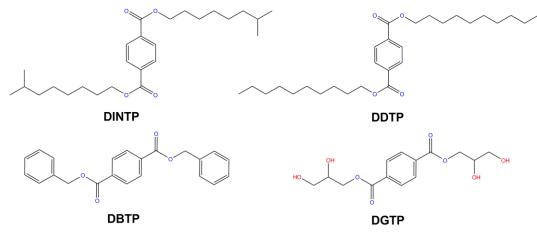
Figure 1. Structural formulas of the synthesized DINTP, DDTP, DBTP and DGTP Slika 1. Strukturne formule sintetisanih DINTP, DDTP, DBTP i DGTP
