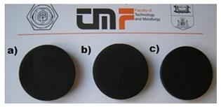
Figure 2.Tested rubber products with a) DINTP, b) DBTP and c) DGTP plasticizer
