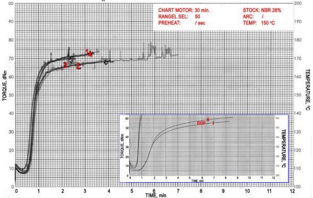
Figure 3. Rheological curves of NBR rubber product based on DOP and PET derived plasticizers Slika 3. Reološke krive NBR gumenih proizvoda baziranih na DOP i PET derivatima plastifikatora
