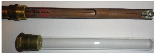
Figure 1. Photo of the hot wire cell used in this work
