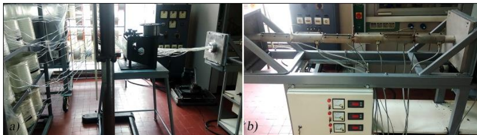
Fig. 1. a) Fiber from the windings on the stand guided to the pultrusion entrance, and b) the pultrusion zones.
