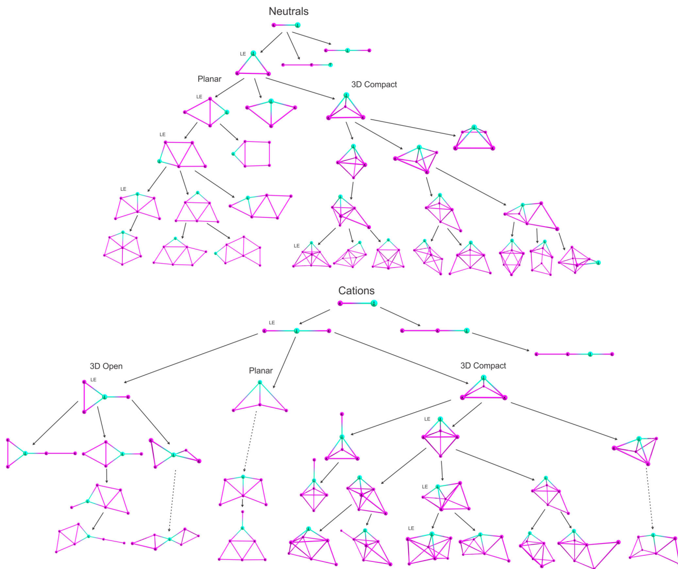
FIGURE 10 Schematic depiction of growth mechanism of K_n I^{(0,+1)} clusters up to the seven atoms
