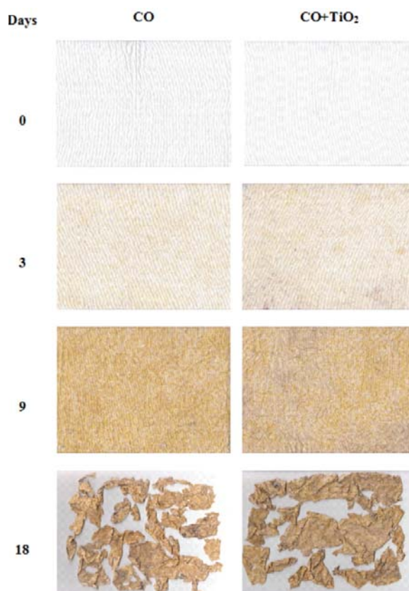
Fig. 4. Photographs of the CO and the CO+TiO 2 fabrics before and after 3, 9 and 18 days of soil burial.
