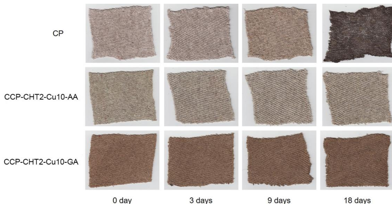
Figure 11. Photographs of studied samples before (0 days) and after 3, 9, and 18 days of soil burial (the sample size: 10 cm × 8 cm).
