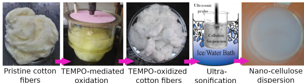
Figure 1. The main steps in obtaining nanocellulose dispersions from TEMPO-oxidized cotton
