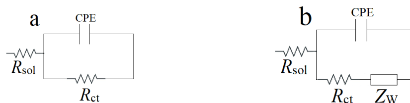
Figure 8. Equivalent circuits used to fit the experimental EIS data: (a) RctCPE and (b) RctCPE-W.
