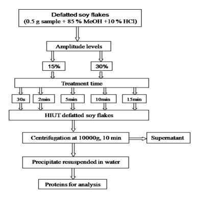
Scheme 1. Schematic representation of an experimental procedure
