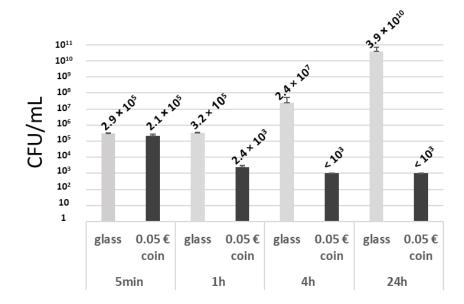
**Figure 2.** Level of surviving bacteria (CFU/mL) after contact during various time periods (5 min, 1 h, 4 h and 24 h) with the negative control glass surface (light grey) or the 5 cent Euro coin (dark grey) positive control.
