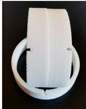
Fig. 2 PRNT specimens fabricated from PA12 material.
