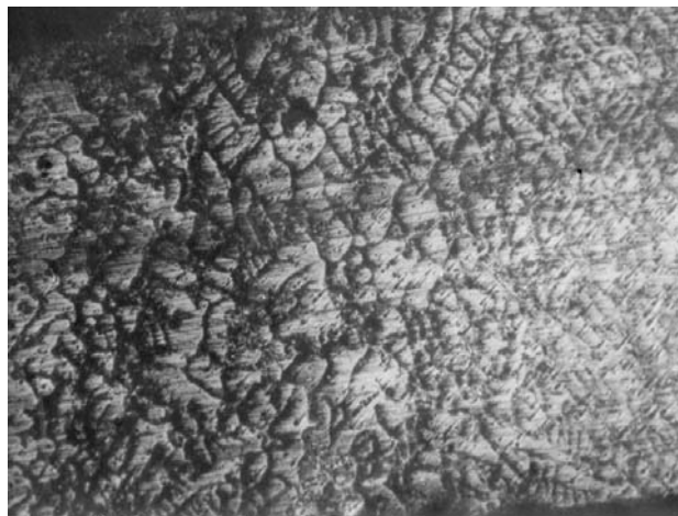
Fig. 1 - The cellular structure. Magification 24x
