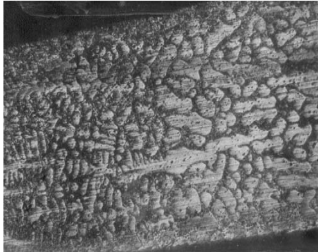
Fig. 2 - Transition from the cellular to dendritic structure. Magification 24x
