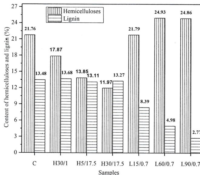
**Figure 1.** Content of hemicelluloses and lignin in unmodified and chemically modified jute fabrics
