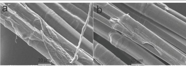
Fig. 2. SEM photographs of control (a) and flax fibers treated with 4% H<sub>2</sub>O<sub>2</sub> at 50 °C (b)
