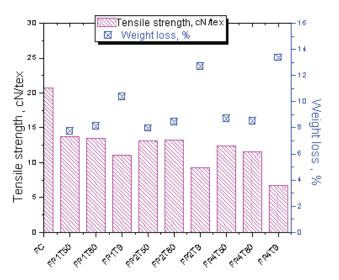
Fig. 5. Weight loss and tensile strength of the unmodified flax fibers and flax fibers modified with hydrogen peroxide
