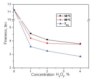
Fig. 3. Effect of the modification conditions on the fineness of flax fibers
