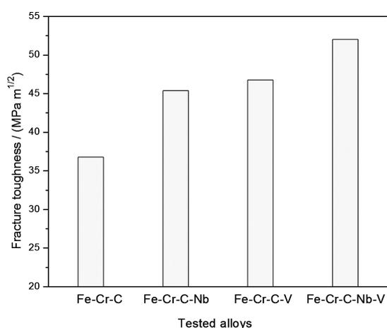
**Figure 9:** Dynamic fracture toughness of the tested alloys
