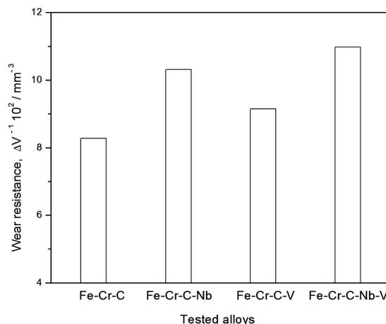
Figure 8: Wear resistance of the tested alloys
