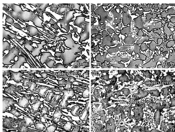
**Figure 1:** LM micrographs of the: a) basic Fe-Cr-C alloy, b) Fe-Cr-C-Nb alloy containing 1.58 % Nb, c) Fe-Cr-C-V alloy containing 1.55 % V and d) Fe-Cr-C-Nb-V alloy containing 1.53 % Nb and 1.47 % V
