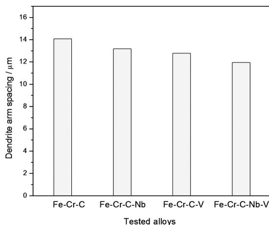
**Figure 5:** Dendrite arm spacing in the tested alloys
