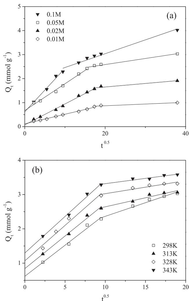
**Figure 6** Plots of IPD model for Mo(VI) sorption on PGME-deta at pH = 2 for: (a) different initial concentrations at 298 K,  $t = 24$  h and (b) different temperatures for  $C_i = 0.1$  M,  $t = 360$  min.
