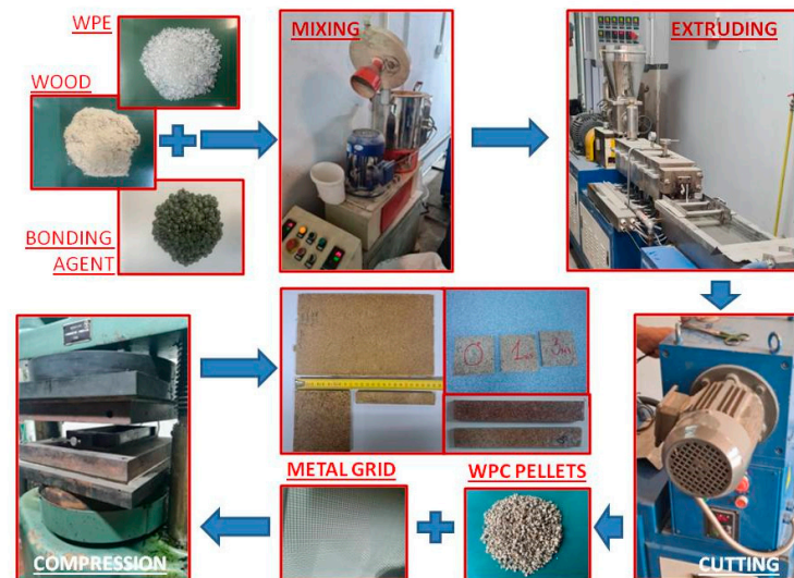
Figure 2. Processing route of WPC materials.
