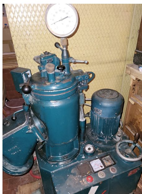
Figure 2. Laboratory hot mixer.
