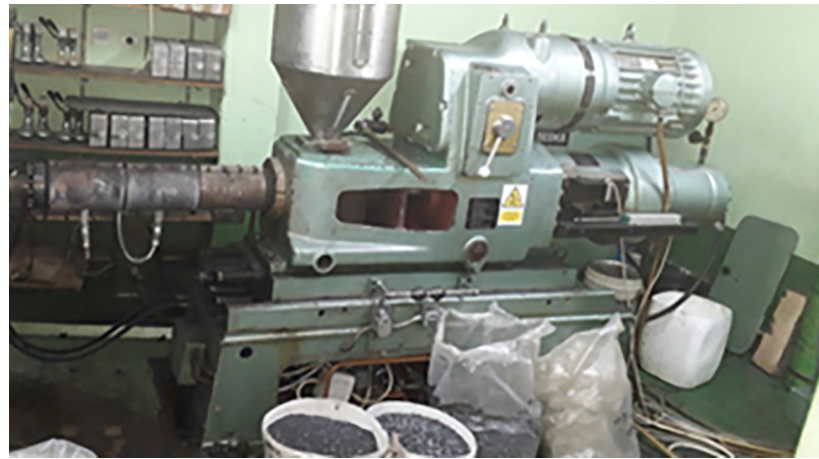
Figure 4. Extruder used for PVC re-granulate processing.
