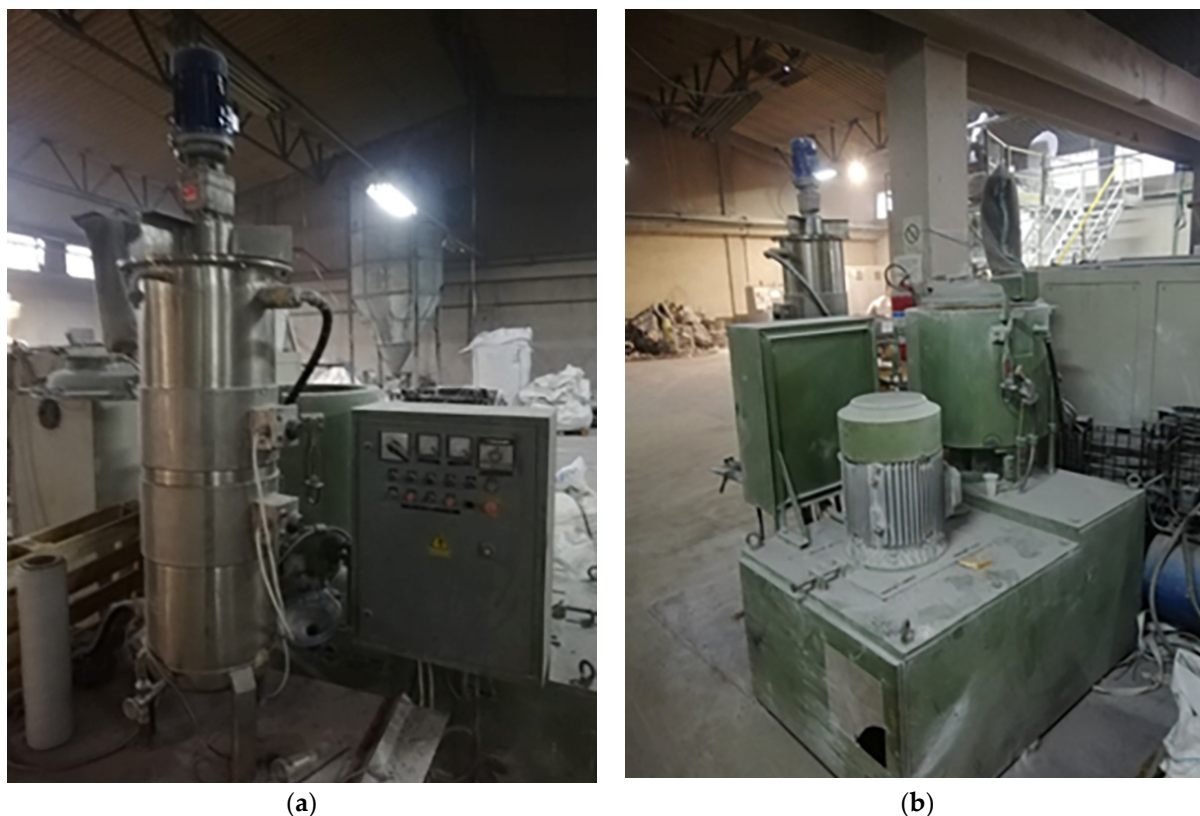
Figure 3. Boiler for controlled heating of hot mixture (a), and hot mixer (b) (PVC high-speed mixer; 50 L) for blending of PVC with plasticizers and additives.
