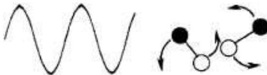
Slika 2. Diopolarni molekuli u oscilatornom električnom polju Figure 2. Dipolar molecules which try to align with an oscillating electric field
