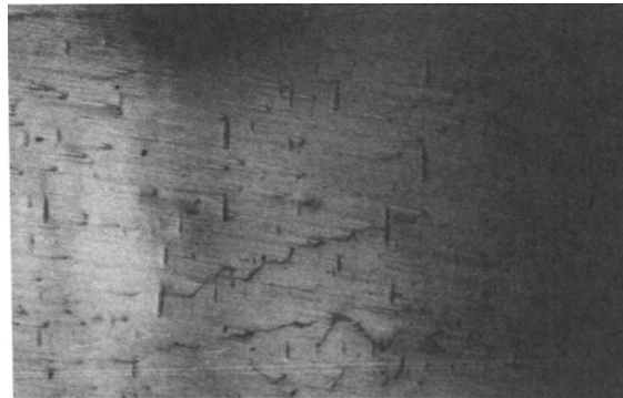
Figure 5. Microstructure of sample solidified with R=8.71 \times 10^{-3} cm/s, irregular cells (magnification \times 24 )
