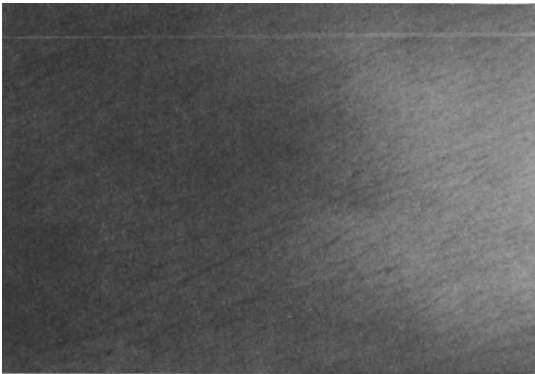
Figure 1. Microstructure of sample solidified with R = 1.45 \times 10^{-4} cm/s, interface – planar (magnification x 24)
