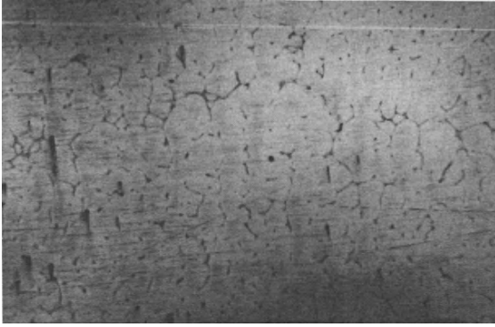
Figure 4. Microstructure of sample solidified with R=8.71 \times 10^{-4} cm/s, beginning of the connection of the cells (magnification \times 24 )
