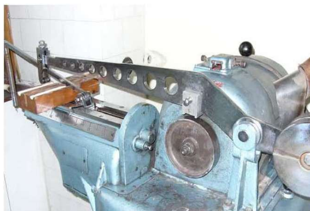
Fig. 3. Tribological and Wear resistance testing device.
