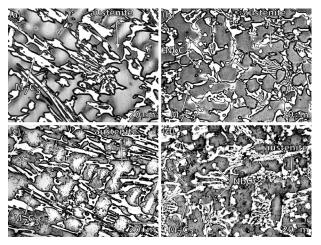
**Figure 1:** LM micrographs of the: a) basic Fe-Cr-C alloy, b) Fe-Cr-C-Nb alloy containing 1.58 % Nb, c) Fe-Cr-C-V alloy containing 1.55 % V and d) Fe-Cr-C-Nb-V alloy containing 1.53 % Nb and 1.47 % V
