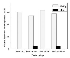
Figure 4: Volume fractions of carbide phases in the tested alloys Slika 4: Volumenski deleži karbidnih faz v preizkusnih zlitinah
