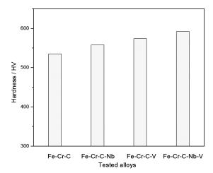
**Figure 7:** Hardness of the tested alloys **Slika 7:** Trdota preizkusnih zlitin
