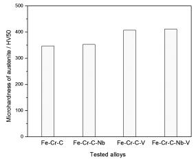
**Figure 6:** Microhardness of the tested alloys **Slika 6:** Mikrotrdota preizkusnih zlitin
