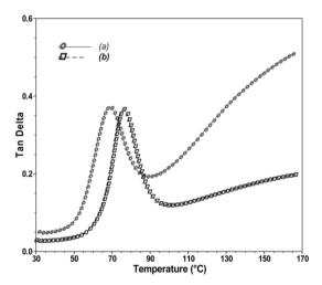
Figure 6 - Tan Delta (tan  $\delta$ ) of: (a) p-aramid/PVB fabrics and (b) p-aramid/PVB fabrics with PVB/SiO<sub>2</sub> nanofibers
