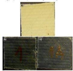
Figure 14 - Samples before the impact test: a) Colon/PVB; b) Colon/PVB/1 wt.% MWCNT; c) Colon/AMEO/PVB/ 1 wt.% MWCNT
