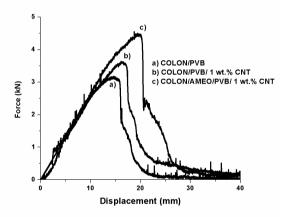
Figure 19 - Force versus displacement for different Colon/PVB fabrics
