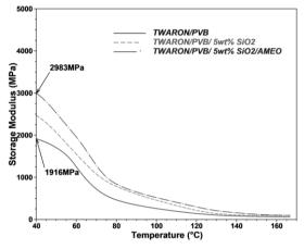
Figure 9 - Storage modulus of the samples
