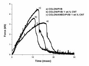
Figure 18 - Force versus time for all the samples
