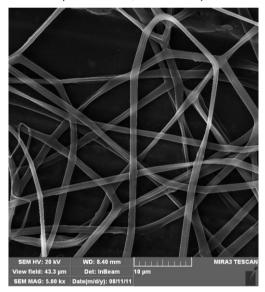
Figure 8 - SEM image of the PVB fibers with 5 wt.% modified SiO<sub>2</sub> nanoparticles (Q = 1 mL/h, V = 30 kV)
