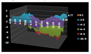
Figure 13 - Indentation depth analysis of the shot No. 1
