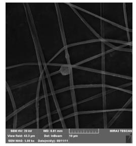
Figure 7 - SEM image of the PVB fibers with 5 wt.% unmodified SiO<sub>2</sub> nanoparticles (Q = 1 mL/h, V = 30 kV)
