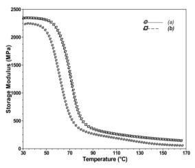
Figure 5 - Storage modulus of: (a) p-aramid/PVB fabrics and (b) p-aramid/PVB fabrics with PVB/SiO<sub>2</sub> nanofibers
