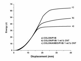
Figure 21 - Energy versus displacement for different Colon/PVB fabrics
