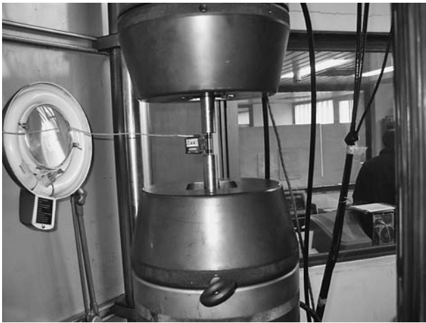
Figure 1 MTS extensometer during fatigue loading
