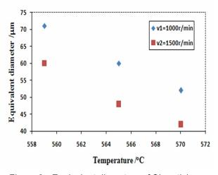
Figure 2 - Equivalent diameters of Si particles versus temperature
