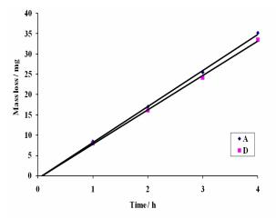
Figure 4 - Cavitation erosion of tested samples as a function of time
