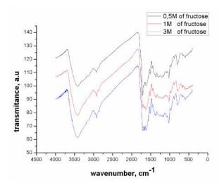
Figure 3 - FTIR spectra of the carbon microspheres obtained by hydrothermal treatment of fructose
