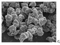
Figure 1 - SEM micrographs of the carbon microspheres obtained by hydrothermal treatment of fructose at 140°C for 3h: a) CMS1; bar length 20μm, b) CMS2; bar length 50μm and c) CMS3; bar length 20μm
