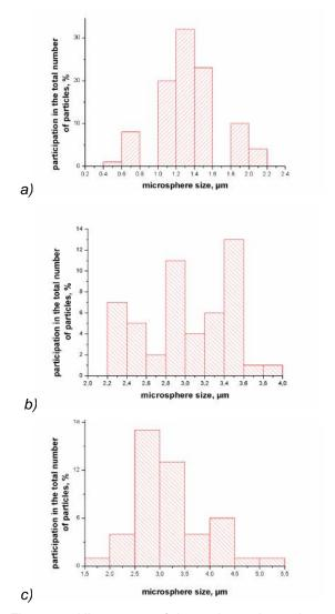
Figure 2 - Histograms of the carbon microspheres: a) CMS1, b) CMS2 and c) CMS3
