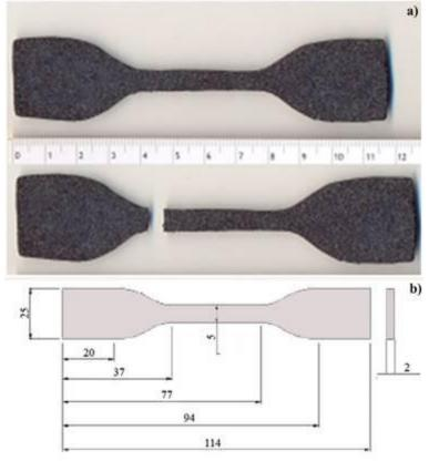
Figure 1. a) Bell shaped specimen for tensile strength testing and b) Schematic presentation of dimensions of specimen
