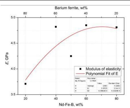
Figure 5. The modulus of elasticity in the function of magnetic medium content in composite materials with 10 wt.% of epoxy resin
