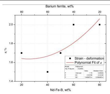
Figure 4. Deformation at the maximum stress in the function of magnetic medium content in composite materials with 10 wt.% of epoxy resin
