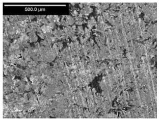
Figure 2. SEM micrographs of Nd-Fe-B-barium ferrite epoxy composite materials ("A" - Nd-Fe-B particles, "B" – barium ferrite agglomerates, "C" – epoxy resin, "D" – smallest particles between large particles and epoxy resin)
