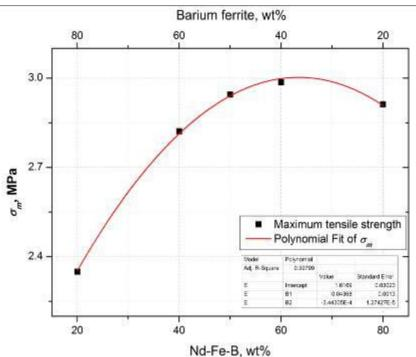
Figure 3 . The maximum stress in the function of magnetic medium content in composite materials with 10 wt.% of epoxy resin
