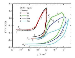
Figure 3. Polarization curve ( $v = 1 \text{ mV s}^{-1}$ ) of aluminum alloy in pH = 7 for different concentrations of sodium chloride ( $E_{corr}$  corrosion potential,  $E_{rp}$ -potential of repassivation or protective potential,  $E_p$ -pitting potential,  $j_p$ -pitting current density)
