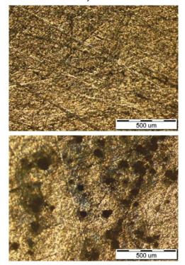
Figure 9. Micrograph images of the aluminum alloy before and after the experiment shown in Figure 8
