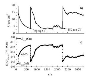
Figure 10. a) The time dependence of the polarization of the aluminum alloy electrode in connection with the copper of an equal surface area without and with the addition of 30 and 180 mg dm<sup>-3</sup> of chloride. b) The time dependence of the corrosion current of the copper-aluminum cell.
