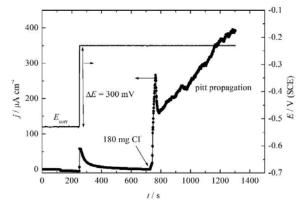
Figure 8. Dependence of the current density over 200 s without chloride, on the corrosion potential, after electrode polarization anodicaly for 300 mV (200-700 s) without the presence of chloride and after the addition of 180 mg dm<sup>-3</sup> of chloride
