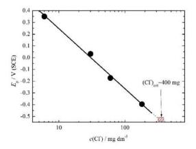
Figure 6. The dependence of critical pitting potential on the concentration of chloride ion. (Cl-)<sub>crit</sub> critical concentration of chloride ion to reach the pitting already on the corrosion potential of ~ -0.55
