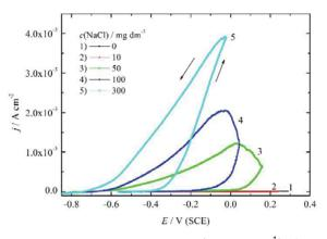
Figure 2. Polarization curve ( $v = 1 \text{ mV s}^{-1}$ ) of aluminum alloy in solution pH = 7 for different concentrations of sodium chloride
