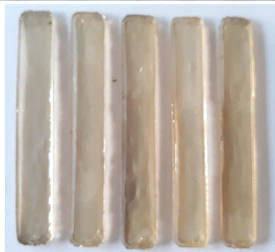
Figure 3. Tube specimens of pure polyester resin (PR) for testing mechanical properties.
