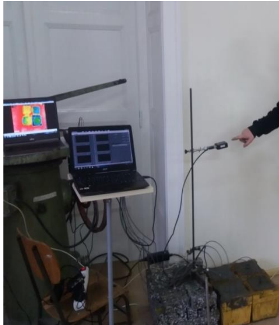
Figure 1 – Experimental setup for the monitoring of heat of hydration of cement
