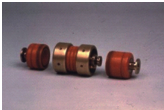
Figure 2. The gas surge arrester gas chamber model
