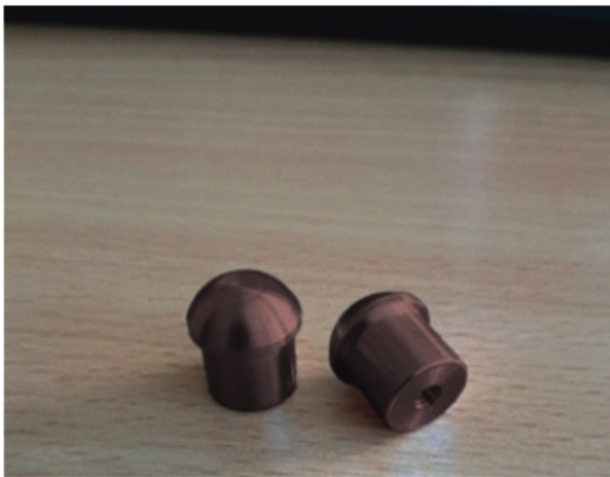
Figure 5. The basic electrodes Rogowski type used in the experiment
