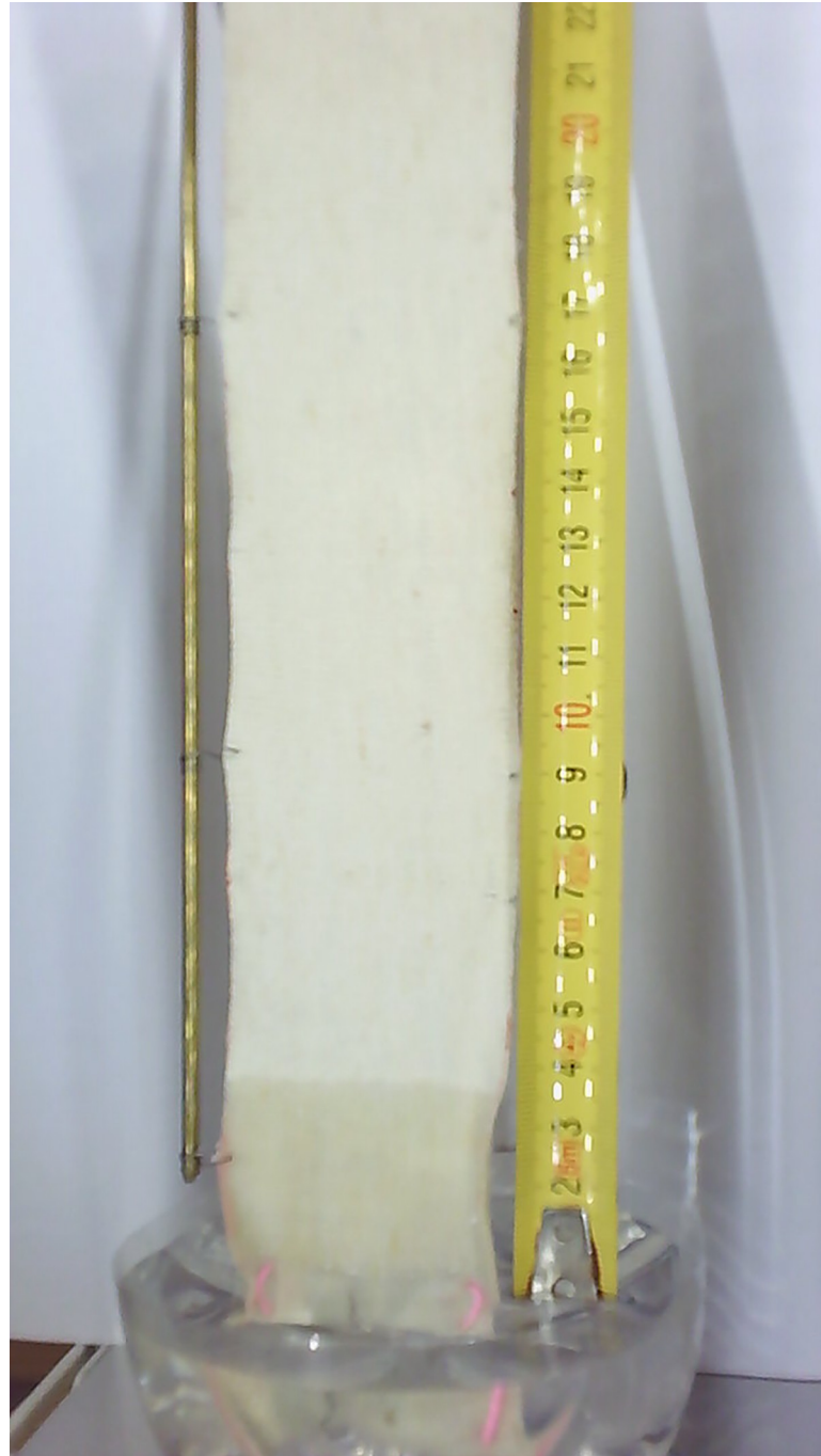
Fig 2. Example of the recorded image during determination of wicking of the hemp knitted fabric.
