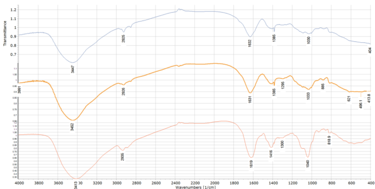
Figure 2. FT-IR spectra of investigated sample: (-) pure alginate beads ( blue line ); (-) activated alginate beads ( orange thick line ); and (-) immobilized alcalase-alginate beads ( orange thin line ).
