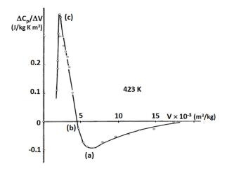
**Figure 10**.  $\Delta C_{p}/\Delta V$  versus volume of ethylene gas at 423 K, drawn according to numerical differentiation of tabulated data [5]. The values of volumes at inflection points (a) and (c) and maximum (b) in Figure 9 can be estimated.
