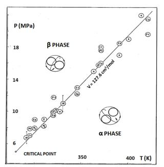
**Figure 15.** P-T coordinates of the marked changes of ethylene properties are situated close to predicted  $\alpha$ - $\beta$  phase transition at critical isochore V = V<sub>c</sub> = 127.6 cm<sup>3</sup>/mol [4].
