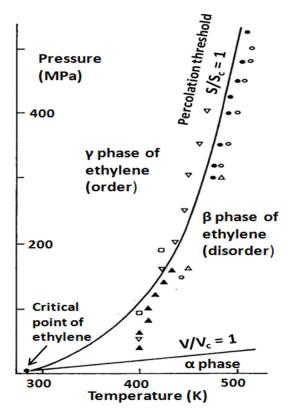
Figure 21. Phase changes in pure ethylene (percolation threshold line S/Sc = 1) and in pure polyethylene (points) occur at the same pressure-temperature conditions. (References for polyethylene melting at high pressure are in [4,29,30].)
