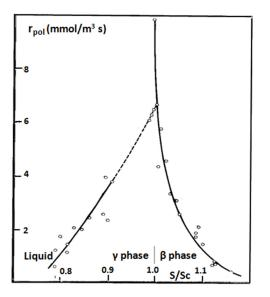
**Figure 18**. Correlation of rate of polymerization  $(r_{pol})$  with reduced entropy (S/Sc) [13,36]. Based on the data [44] on temperature and pressure under polymerization conditions we have read reduced entropy using the diagram [26] and correlated it with  $r_{pol}$ .
