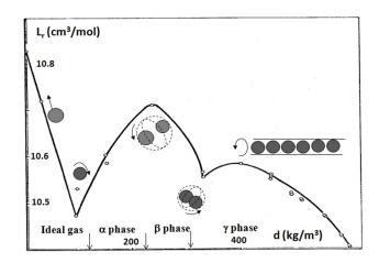
**Figure 16**. Lorentz-Lorenz function  $L_r$  (molar refraction) as a function of ethylene density at 298 K. Maximal errors of  $L_r$  are in the range 0.015-0.040 (from Table III in [33]). We denoted the predicted phase transition conditions ( $\downarrow$ ) and type of supramolecular species.
