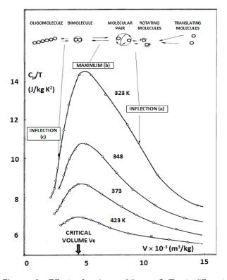
**Figure 9.** Effect of volume (V) on  $C_p/T$  at different temperatures, drawn according to data [5]. Inflection (a), maximum (b) and inflection (c) are denoted on the curves as well as corresponding phase transitions of compressed ethylene gas.
