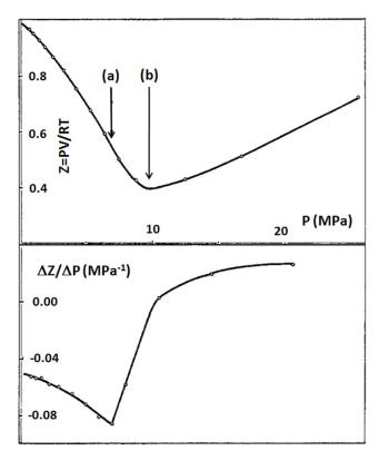
**Figure 13**. Effect of pressure P on the compressibility factor Z (upper) and derivation  $\Delta Z/\Delta P$  (bottom) at 313 K. Based on numerical data in [1,31].
