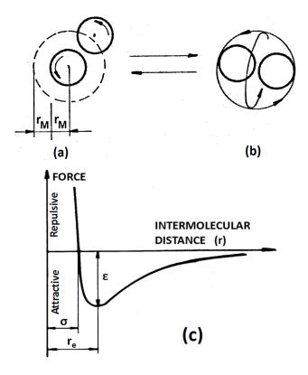
**Figure 3**. (a) Restriction of free rotation of single molecules; (b) Formation of molecular pair; (c) General shape of Lennard-Jones's potential [8]. For ethylene: s = 0.4163 nm and  $r_e = 0.466$  nm [9].
