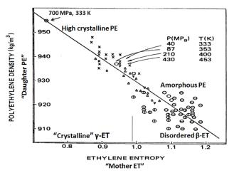
**Figure 20**. Effect ET entropy under polymerization conditions on PE density [4,29].
