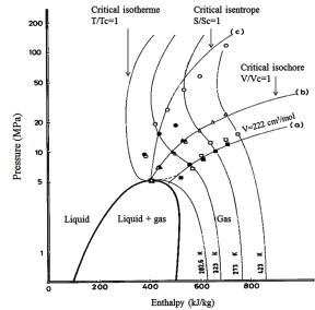
**Figure 11.** Positions of the maxima (triangles) and the inflection points (circles and squares) on  $C_p$  (open symbols) and  $C_v$  (filled symbols) curves drawn onto enthalpy-pressure diagram [26] of ethylene.
