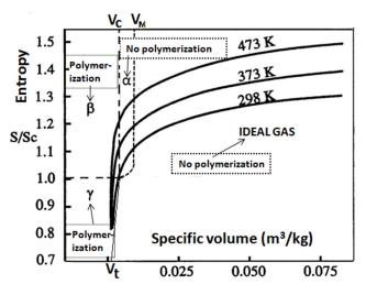
**Figure 17**. Dependence of reduced entropy on the volume of ethylene [4,13,36] based on [26]. Phase states are denoted according to Figure 12.
