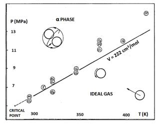
Figure 14. P-T coordinates of the marked changes of ethylene properties are situated close to predicted ideal gas to  $\alpha$  phase transition at isochore V=222 cm<sup>3</sup>/mol [4].
