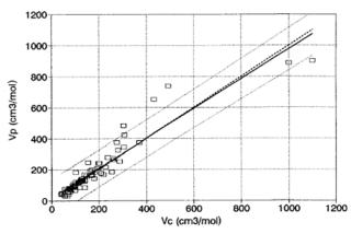
**Figure 22.** Volumes of molecular pairs V<sub>p</sub> calculated by Eq. 3 are equal to the empirical values of critical volumes V<sub>c</sub> [53].  $\Box$  empirical data; — Regression; ---- Expected; ..... Confidence limits. Standard error is 60.1 cm<sup>3</sup>/mol; Correlation coefficient 0.94. (Based on the empirical data [9] for 92 substances for r<sub>e</sub> and V<sub>c</sub>).
