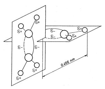
Figure 4. Configuration of a molecular pair [3,4,12,13].
