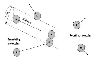
Figure 2. Restriction of free translation and formation of rotating single molecules by collision of two translating molecules.
