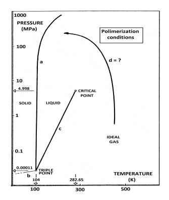
**Figure 1**. Pressure-temperature diagram for ethylene, drawn according to data [1,5]. Critical point:  $T_c$ =282.65 K, P\_c=5.06 MPa, V\_c=127.64 cm<sup>3</sup>/mol; Triple point:  $T_t$ =104 K, P\_c=111.5 Pa, V\_c=39.08 cm<sup>3</sup>/mol.
