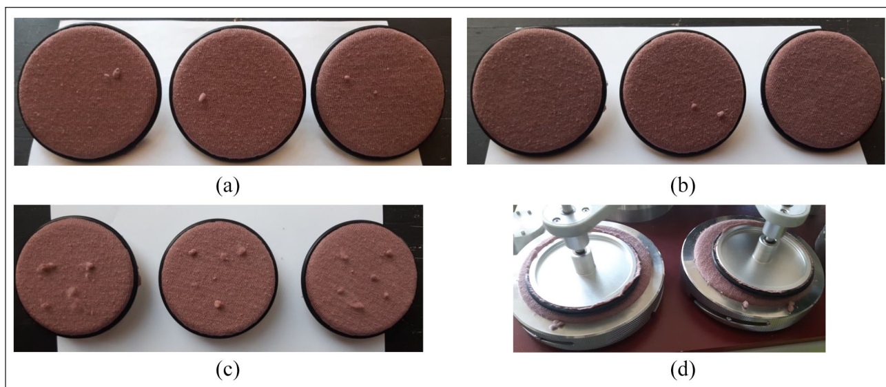
Figure 3. Appearance of Sample 3: after (a) 2000, (b) 5000, (c) 7000 rubs, and (d) removal of the pills during abrasion.
