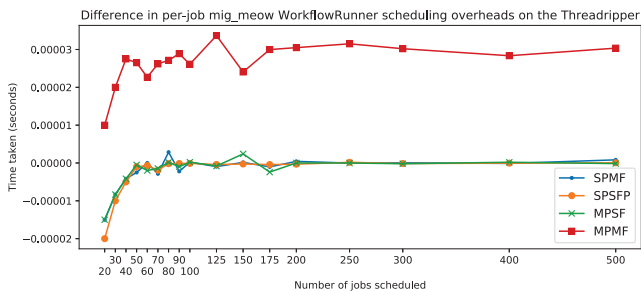
Fig. 8. Delta in per-job WorkflowRunner scheduling durations on the Threadripper. Note that the SPSFS result have been excluded as it has a much greater scale that crushes the rest of the results.
