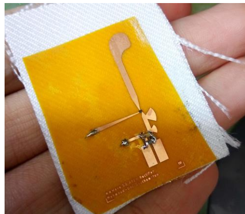
Fig. 3. Prv-Si tandem cell spectral response [13] Fig. 4. Rectenna harvesting \lambda=1\text{mm} waves
