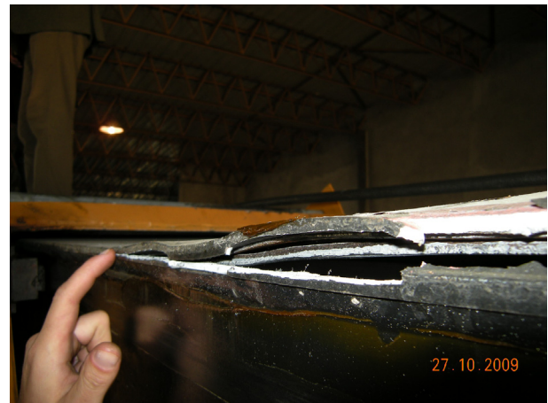
Figure 2 Deformation and cracks on steel construction of vehicle-mounted crane
