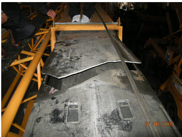
Figure 1 Crack of telescopic arm of vehicle-mounted crane
