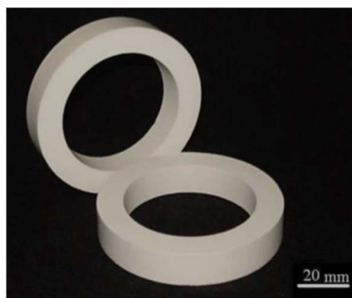
Fig. 8. Ceramic set of rings for sealing used in pumps for transport of fluid with outer and inner diameters of 63 mm and 51 mm, respectively.
